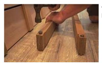
Tap the Provided (4) – "T-Nuts" into the holes on the bottom of the 2 side staves with a hammer.
