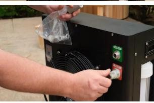
Install the inlet filter onto the inlet connection.
