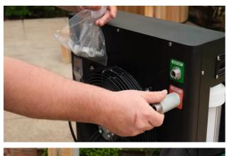
Thread the Filter guard over the inlet filter.
