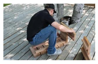
To assemble the 2-tier step (if ordered), place the top step upside down and a stair support on top.
