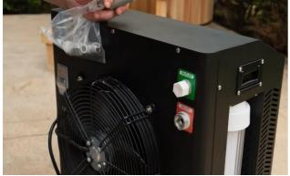
Remove the covers on the inlet and outlet on the back of the chiller.
