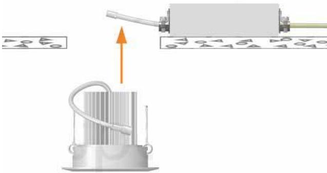
If you ever need to remove the light in order to access your driver box, simply grab hold of the sides of the light and gently pull downwards until the light comes about 1/2" down out of the hole. Before pulling the light all the way out of the hole, be sure to get a firm grip on the retention clips, so you can hold them upwards in order to avoid them snapping closed. Then, pull the light the rest of the way out of the hole and gently let the retention clips back down.
