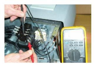
The timer is broken down into two sections. These sections are 1 with 1A and the other section is the number 2 with 2A. Both 1 and 2 are power feeding into to the timer where as 1A and 2A are the power out terminals of the timer.
