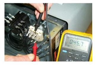
Terminal 11 should read continuity with 21, terminal 12 should read continuity with 22 and 13 should read continuity with 23.
